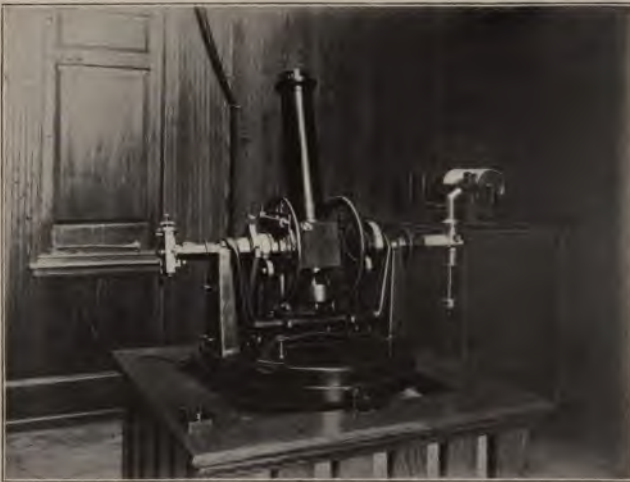
FIG. 52.—A combined transit instrument and zenith telescope.
